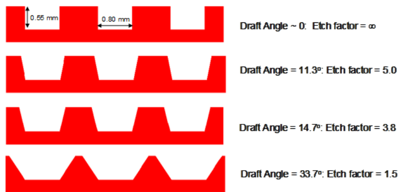
Figure 3.3. Geometries with four different draft angles used in this study. Note that the standard channel shape in this study is ~0 draft angle.
